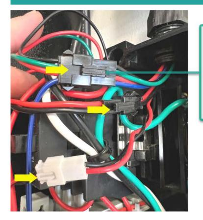
Step 5: Connect the Installed Wires to the MagSwitch Device.
