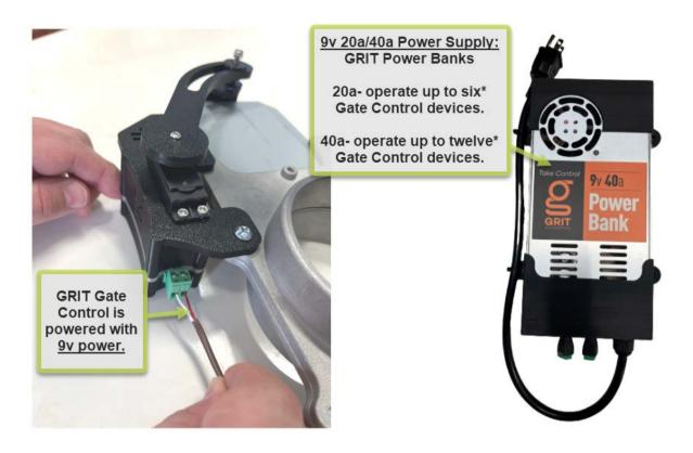
The low-voltage wire can be run from a device to the Power Bank in a "home run" fashion, or, hopped from one Gate Control device to the next on its way to the Power Bank in a "daisy chained" fashion. The Power Bank has two low-voltage jacks, but two sets of wires can be landed in each, if needed.
