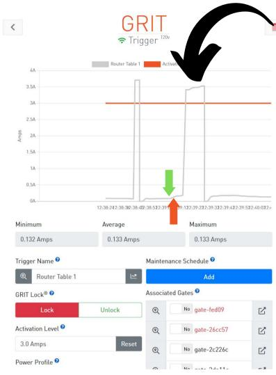
The second spike on the graph was captured with a Normal power profile setting. The green arrow shows when the tool was turned on, the orange arrow indicates when GRIT checks whether the tool is pulling power above the set Activation Level.
