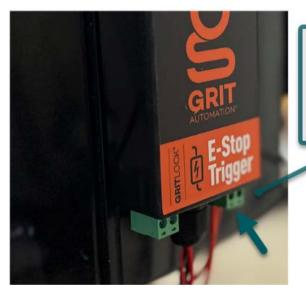
Plug the E-Stop Contact green terminal back into the bottom right-hand side of the E-Stop Trigger. Triggers Installation
